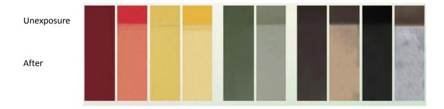
Test wall at Taiyo Steel Works, Japan 1981-1995
